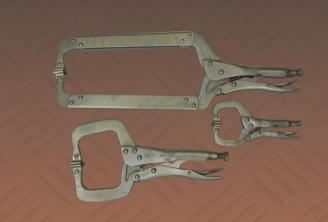
**Locking C-Clamp** made from high grade alloy tool steel, heat treated for maximum hardness, powerful locking mechanism, wide opening C shaped jaws, knurled pressure adjustment screw, and guarded release
