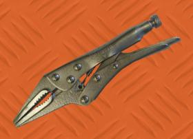
**Locking Pliers** made from high grade alloy tool steel, heat treated for maximum hardness, powerful locking mechanism, curved jaws allow user to put pressure on 4 points of any nut or bolt, precision cut teeth, built in wire cutters, knurled pressure adjustment screw, and guarded release
