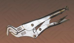
**Locking Pliers** made from high grade alloy tool steel, heat treated for maximum hardness, powerful locking mechanism, curved jaws allow user to put pressure on 4 points of any nut or bolt, precision cut teeth, built in wire cutters, knurled pressure adjustment screw, guarded release, and large Sure-Grip handles
