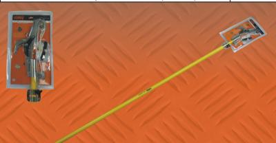
POLE PRUNER - Fiberglass Handle 12"High Speed Steel saw blade, cross cut Gator-Tooth™ blade cuts 2X as fast as normal blades, non-stick coated lopping blade, heavy duty all steel housing, 132" maximum reach telescopic lightweight fiberglass poles, fiberglass poles are shockproof for extra safety when working close to power lines
