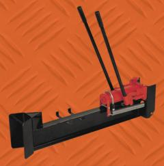
**10 Ton Hydraulic Log Splitter -** manual splitter will be able to generate up to 10 tons of force splitting logs as long as 18" and as thick as 6-1/2" in diameter, minimum log length is 13-1/2", ram stroke 8-1/16", splitting wedge size is 4"L x 3-3/4"W x 4"H, this splitter will save hours of manual labor
